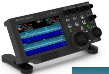
A FlexRadio Maestro (wireless or wired) connects across a local network or the internet to control a FlexRadio station. Can also control from a PC program or App on smartphone or tablet. Remote access has been "built-in" to the SmartSDR software.
