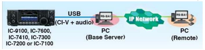
Some models (7800, 7610) direct to IP Network without Base Server. But Base Server useful to control other shack functions (rotators, amplifier,...)
