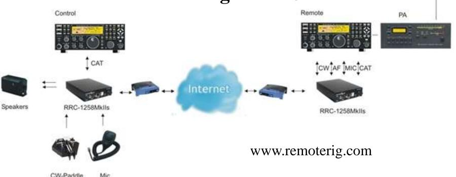
Use a pair of RemoteRig "modems" to send audio and control signals to station. Can use with: detached front panel(TS-480), "control heads" (Elecraft K3/0-Mini), "twin" pair of radios, a PC program or an Android App.
