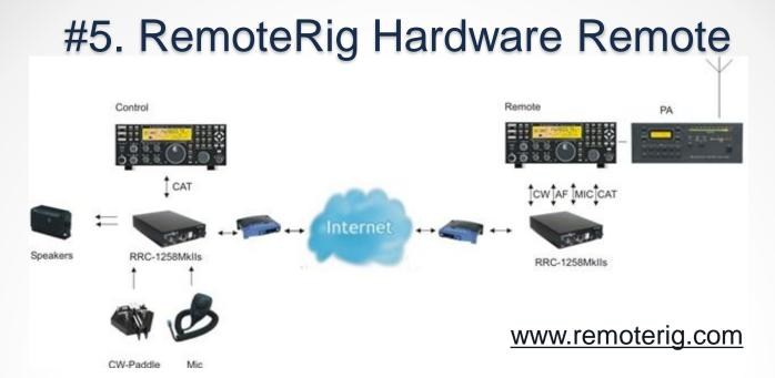
A detachable front-panel, or a 2nd radio in "twin" mode, is used to control the remote radio. The RemoteRig "modems" extend the rig control, audio, keying, serial port, ... No PC required to operate, but needed for initial setup.
