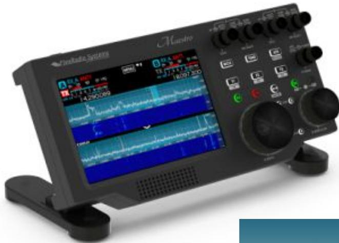
A FlexRadio Maestro (wireless or wired) connects across a local network or the internet to control a FlexRadio station. Can also control from a PC program or App on smartphone or tablet. Remote access has been “built-in” to the SmartSDR software.
